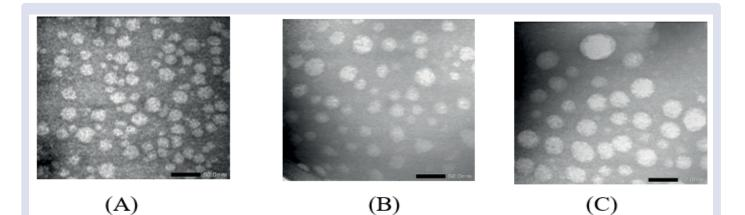
Figure 2: Results of meniran extract nanoparticles (Phyllanthus niruri Linn) using the TEM test. (A) 5%, (B) 10%, (C) 20%.
