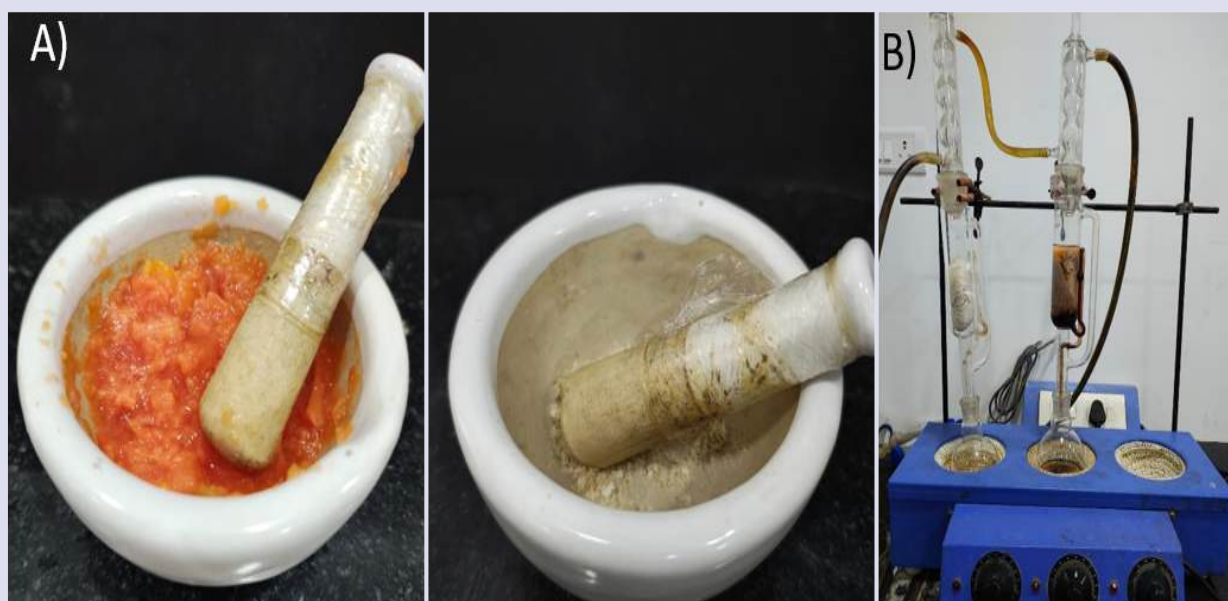
Figure 1. A) Moringa oleifera seed and Carica papaya fruit sample finely ground using mortar and pestle for nanoparticle synthesis. B) Soxhlet extraction of plant materials.
