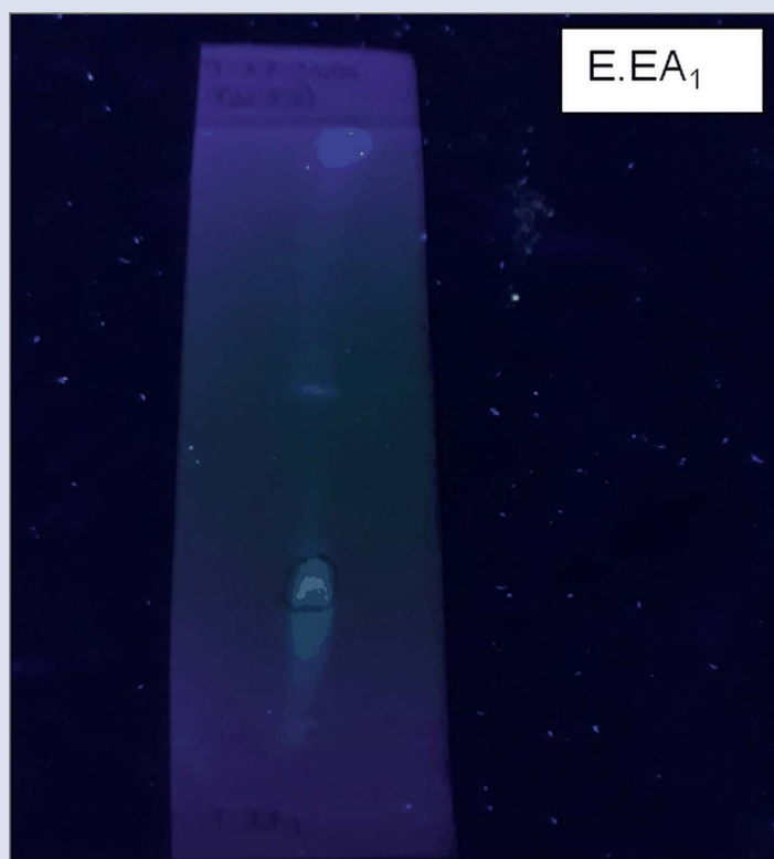
Figure 14. E.EA 1 obtained from ethyl acetate fraction was spotted on TLC plate and developed with toluene: ethyl acetate: methanol (22:8:8) solvent system. TLC plate viewed under UV light.
