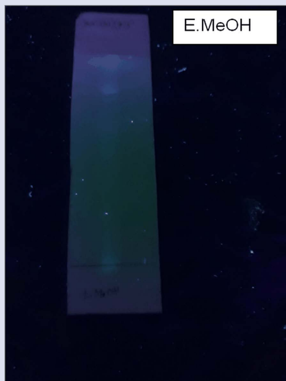
Figure 15. E.MeOH obtained from hydromethanolic fraction was spotted on the TLC plate and developed with n-hexane: chloroform (7:3) solvent system. TLC plate viewed under UV light.
