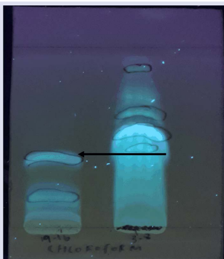
Figure 7. The TLC chromatogram of E. elephantina rhizome chloroform fraction. Fractions 3-6 and 9-16 were collected from the column chromatography and spotted on the TLC plate and developed with ethyl acetate: n -hexane (9:1) solvent system. Reference plate under UV-light.
